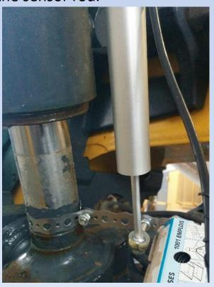
• The sensor will take 24V DC input, and the output Voltage will change when the distance changes. The output voltage will be connected into an AtoD convertor, then connected to the onboard computer via USB port.
